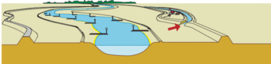
II. River by-pass construction to be used in case of periodic high water levels
