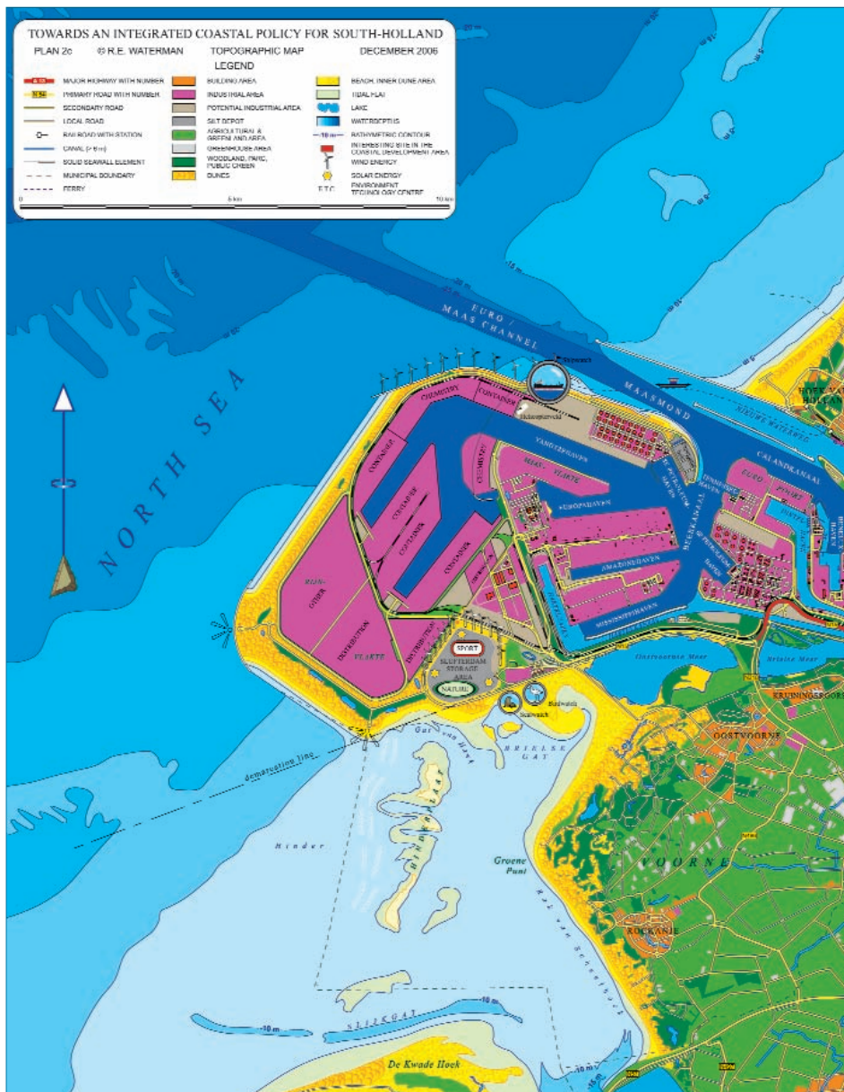
Figure 15. Seaport Marina IJmuiden / Kenemer Beach, Plan 3a. Nature already developed a new area south of the existing southern harbour mole of IJmuiden, owing to littoral sand transport in a northern direction along the coast from the Province of South Holland to the Province of North Holland. The process was quickened by human induced action – dredging external and internal waters. © Ronald Waterman.
