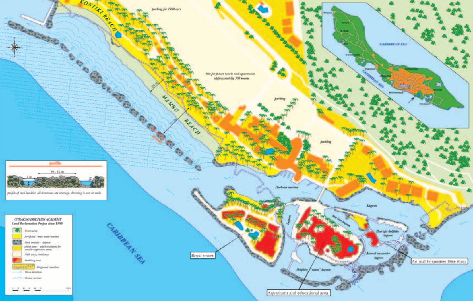
Figure 26. Map of the plan of Curaçao Sea Aquarium land reclamation project, with insert of rock boulder profiles.
