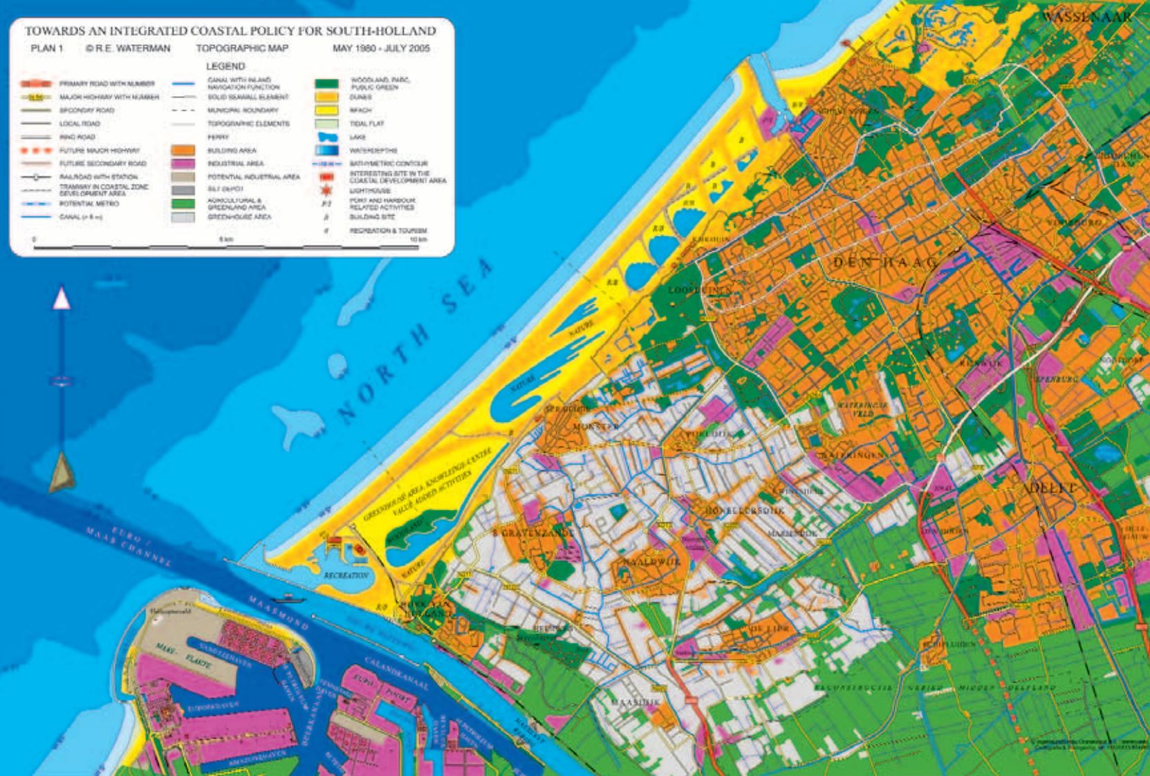
Figure 6. Plan 1 is for a wedge-shaped land reclamation between North Schevevningen and Hoek van Holland, circa 21 km in length and its width is gradually increasing from a few metres near North Schevevningen to approximately 4 km near Hoek van Holland.
